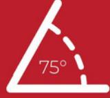
A leaning ladder should be at a 75 degree angle
